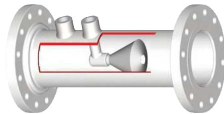
fig.4: V-Cone Flowmeter
